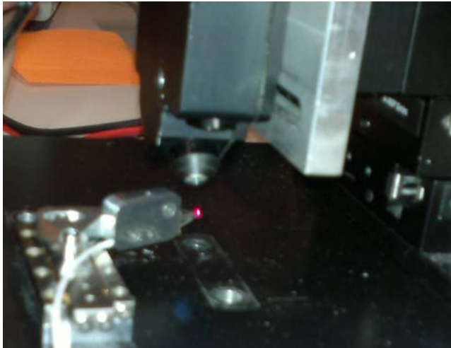
Fig. 8. Microgripper under laser sensor measurement.
